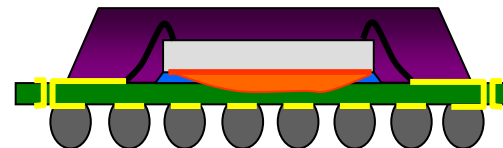
Stage 3: Delamination propagation
